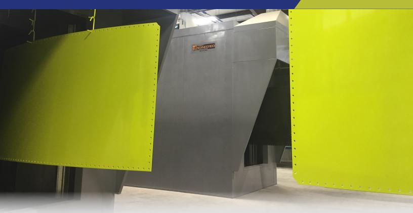
In the next step, tank components are run through a highly efficient gas convection dry-off oven to ensure the tank components are completely dry, preventing flash rusting prior to painting.
